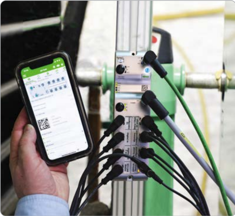
WAGO's System Field distributed I/O modules are sealed to IP67 standards (waterproof when immersed for up to 30 minutes at a depth of one meter) and feature Bluetooth connectivity for local configuration, commissioning and troubleshooting.
