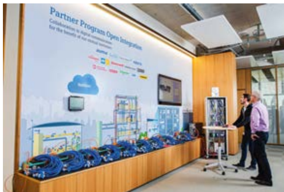
Figure 3: Endress+Hauser load tested an Ethernet-APL network and components by integrating 238 field devices into an Ethernet-APL system at its headquarters in Reinach, Switzerland. It deployed field switches from Pepperl+Fuchs and controls from Honeywell and ABB. The two tests found that Ethernet-APL provided increased bandwidth and speed for easier data access and improved transmission from the field. Source: Endress+Hauser
