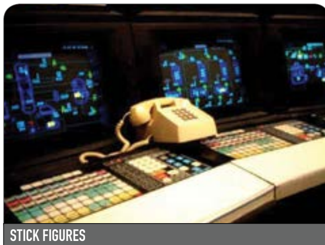
STICK FIGURES FIGURE 3: Initial, DCS-based process representation graphics were crude and fairly low resolution, and their design was based on simple segregation of the plant P&ID.
