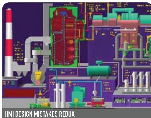
FIGURE 4: A lack of human factor education had led HMI makers to promote 3-D objects that fix more 60% of a screen's data in the foreground, while real data useful for detecting and diagnosing abnormal situations shoved into the remaining 40% of the graphic's background.
