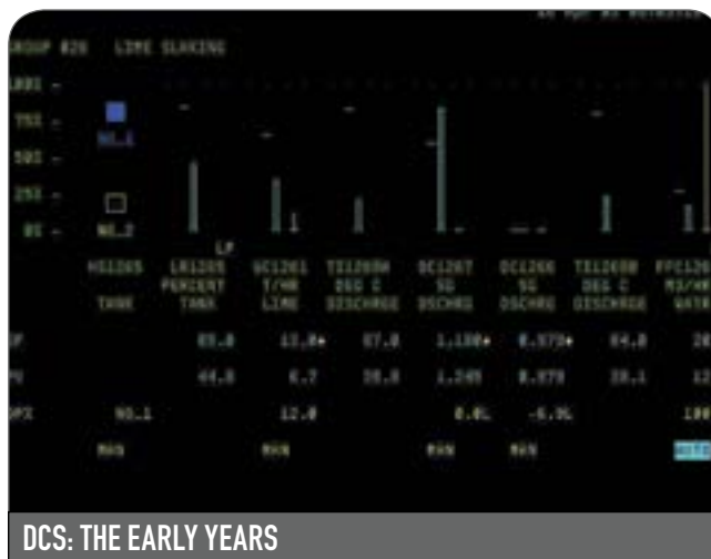
DCS: THE EARLY YEARS FIGURE 2: Originally, DCSs didn’t have an overview feature, and only gave operators access to a group of eight controllers.
