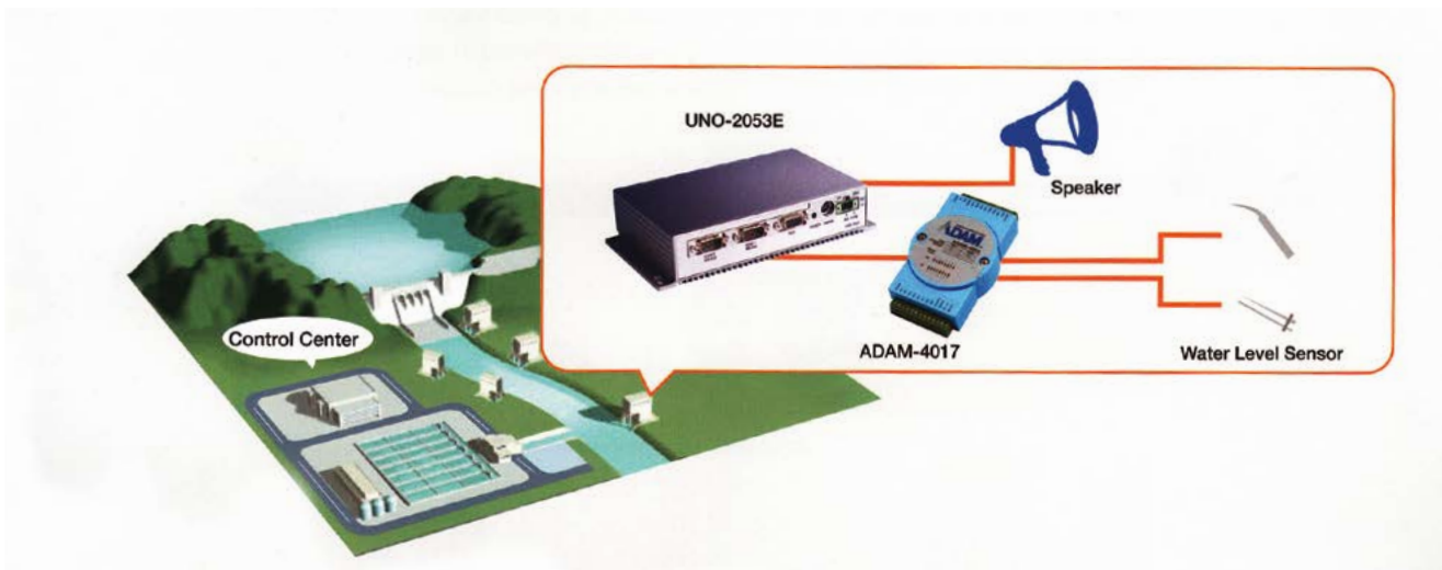
Figure 1. A user performing real-time flood monitoring and alert services is using UNO-2053E and ADAM-4017 to remotely check water-level sensors in Malaysia's rivers, and broadcast warnings when high water levels occur.
