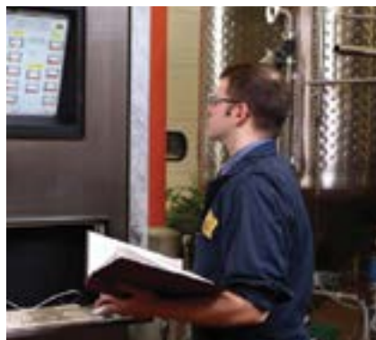
Figure 1: To better control fermentation temperatures, Bell’s Brewery is using Siemens’ Braumat PCS 7 Box, which compresses the functions of a complete DCS into a compact industrial PC platform.
