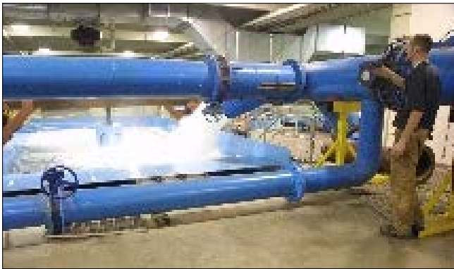
Figure 2. An operator monitors the flow into the 300,000 lb. capacity weight and volumetric calibration water tank at Utah State University's Hydraulics Lab in Logan, Utah.
