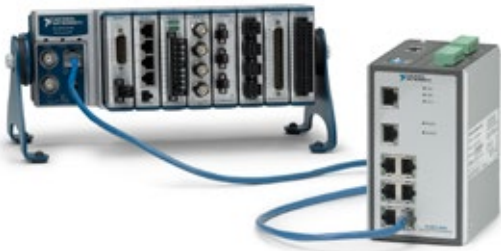
Figure 6. Supporting 100 m per segment and the ability to use existing network infrastructure, Ethernet data acquisition can extend the reach of your measurement system.
