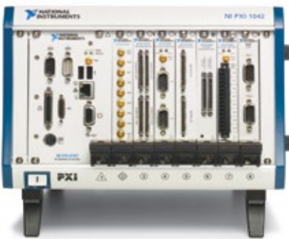
Figure 5. The PXI platform is composed of chassis, controllers, and I/O modules.
