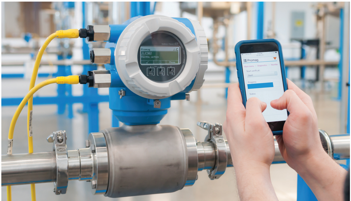
Figure 5: For field verification, a technician connects a smart device to the flowmeter's web server via an optional WLAN connection, up to 15 feet in proximity. The same procedure can be performed via laptop PC and Ethernet connection. The flowmeter does not have to be removed for this procedure
