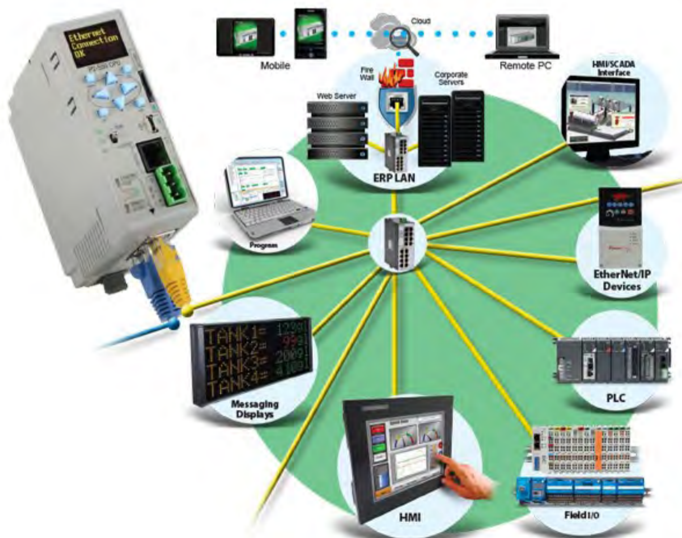
Figure 6A: In an industrial environment, Ethernet is used to network PCs, controllers and other intelligent industrial automation components. Lower level networks are often used to connect controllers to field instruments and sensors.
