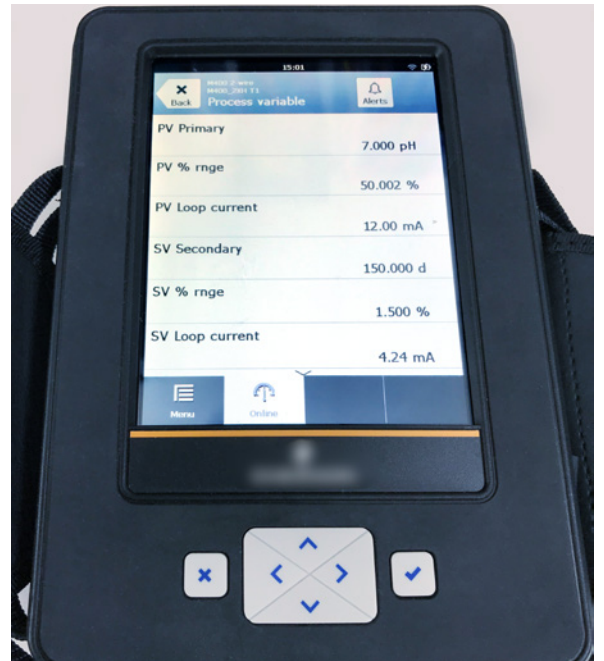
Figure 1: Portable handheld Field Communicator displaying ISM information
