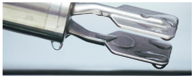
Figure 2: The oscillation of a tuning fork instrument changes when a liquid reaches the two forks.
